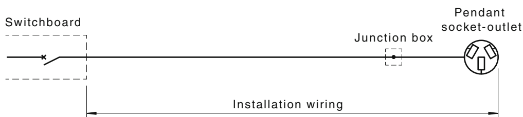
FIGURE 4.8 EQUIPMENT WIRING—EXCEPTION FOR PENDANT SOCKET-OUTLET
